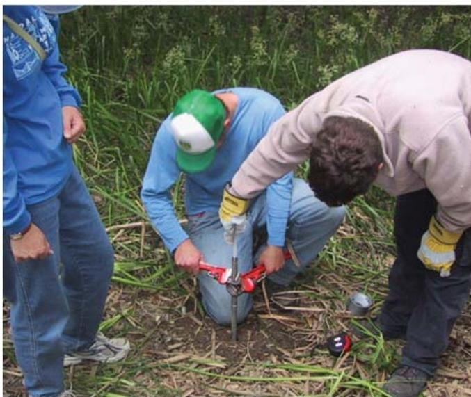
*Installing piezometers to monitor water levels adjacent to Searsville Reservoir.*
